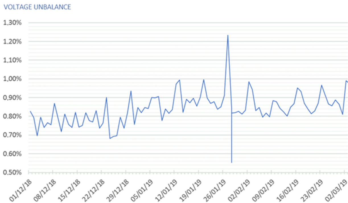
Figure 6. Three-month record of daily maximums of voltage unbalance.
