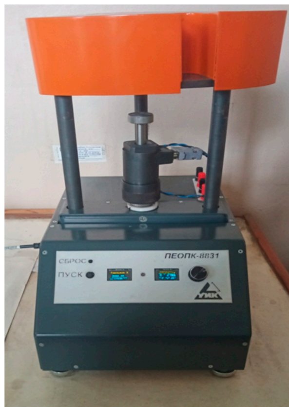
Figure 3. Installation for determination of electrical resistivity.
