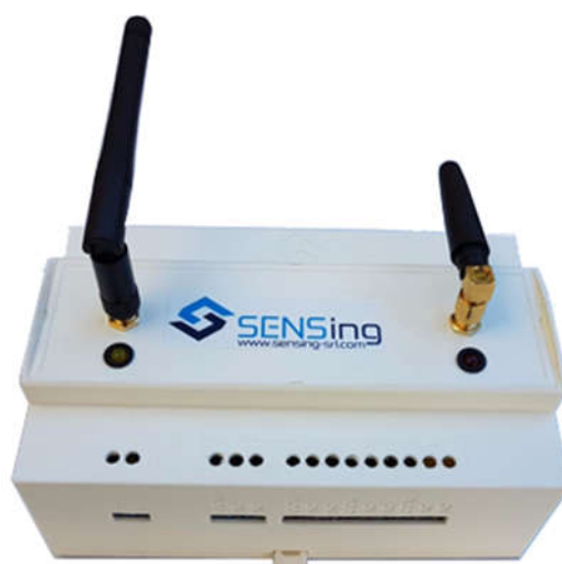
Figure 12. The datalogger prototype (Also for this component external antenna and solar panel can be added).
