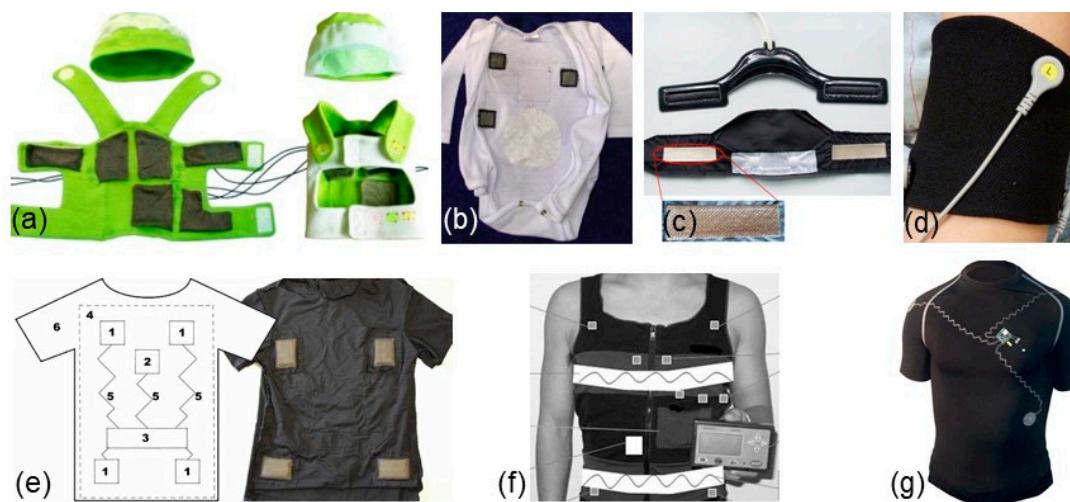
Figure 4. Wearable electrocardiography (ECG) systems: (a) jacket for baby [108]; (b) textile electrodes embedded into a baby suit [109]; (c) belt with embroidered electrodes [59]; (d) armband with embedded textile electrode [69]; (e) Bluetooth-enabled mobile ECG monitoring system integrated on a t-shirt [133]; (f) t-shirt embedded with textile electrodes and a local portable device [110]; (g) t-shirt with embroidered electrodes [134].
