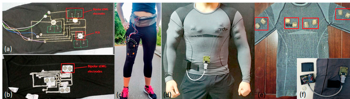
Figure 6. Wearable electromyography (EMG) acquisition garments: running leggings and a sports shirt. Electrode placement in the (a) exterior; and (b) interior of leggings; (c) actual view of leggings when worn by a subject [153]; (d) shirt as worn by a subject; (e) location of electrodes on the shirt; (f) close-up view of the acquisition unit attached to the shirt [115].
