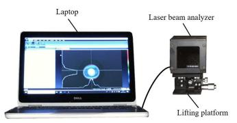
Figure 4. Test equipment of laser beam spot image collection.
