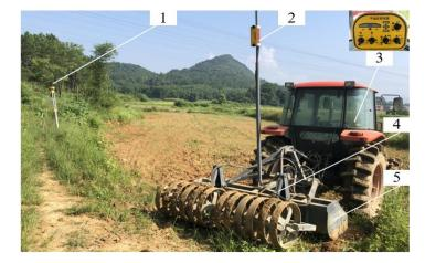
**Figure 10.** Test site of farm levelling. (1. Laser transmitter, 2. Laser receiver, 3. Controller, 4. Hydraulic system, and 5. Scraper.).
