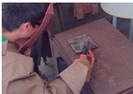
Figure 5. Wearing Safety Protective Gear for Welding.
