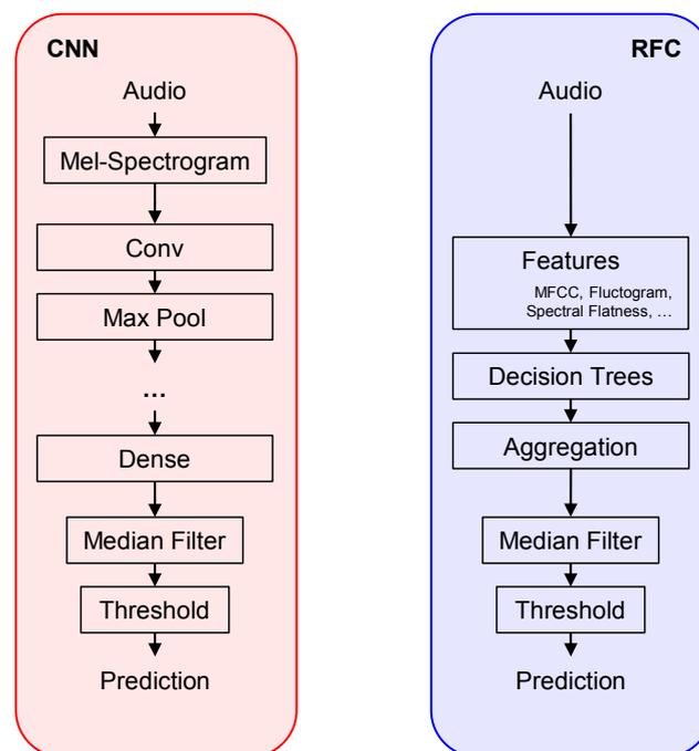
**Figure 1.** Conceptual overview of the two methods for singing voice detection considered in this paper. While the CNN-based approach operates directly on mel-spectrogram excerpts, the RFC requires an additional feature extraction step. Both approaches output continuous predictions which are post-processed using a median filter and thresholding. The exact architecture of the CNN is omitted for brevity. We refer to the original publications for details.
