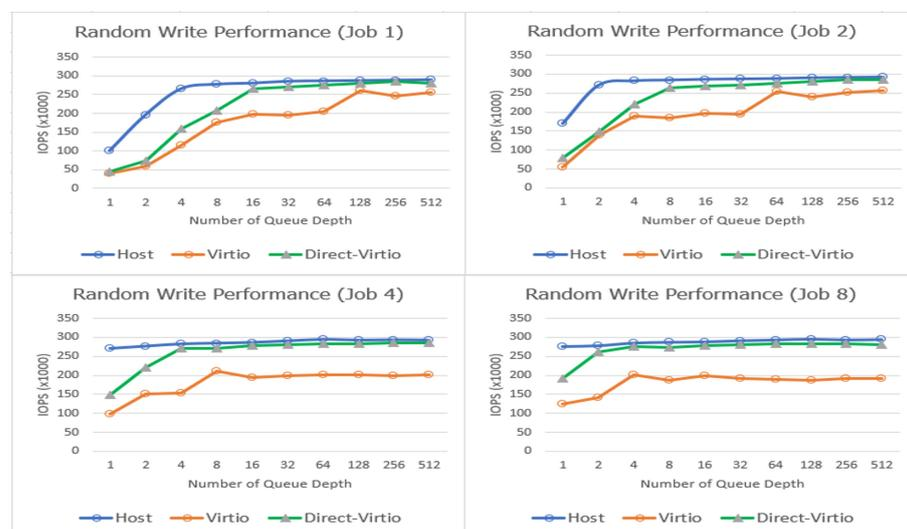
Figure 6. I/O performance comparison between Virtio and Direct-Virtio for random write pattern.
