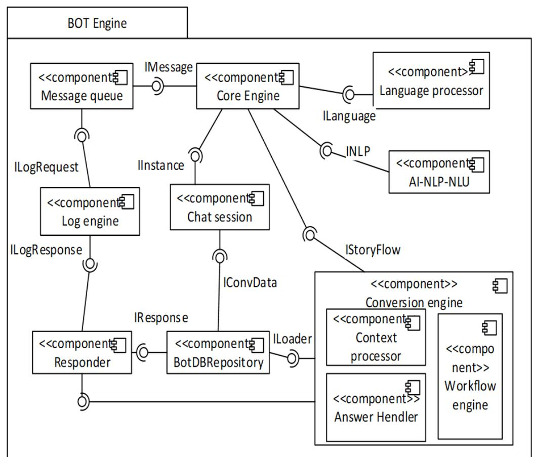
Figure 2. Bot engine component diagram.
