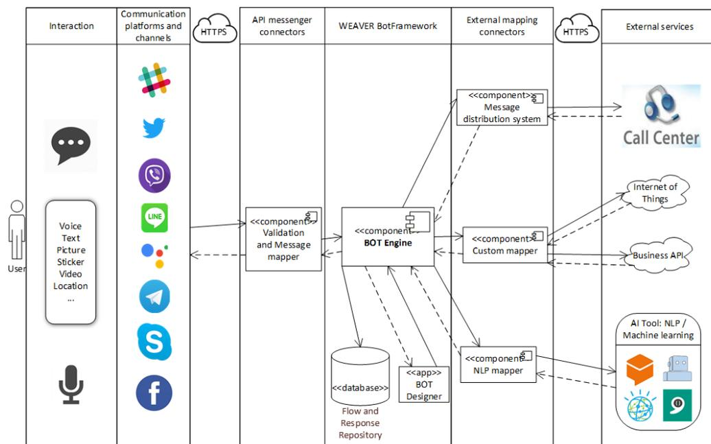
Figure 1. The logical architecture of the proposed solution.
