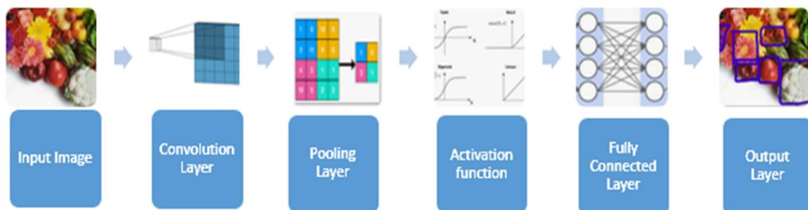
**Figure 2.** CNN components.
