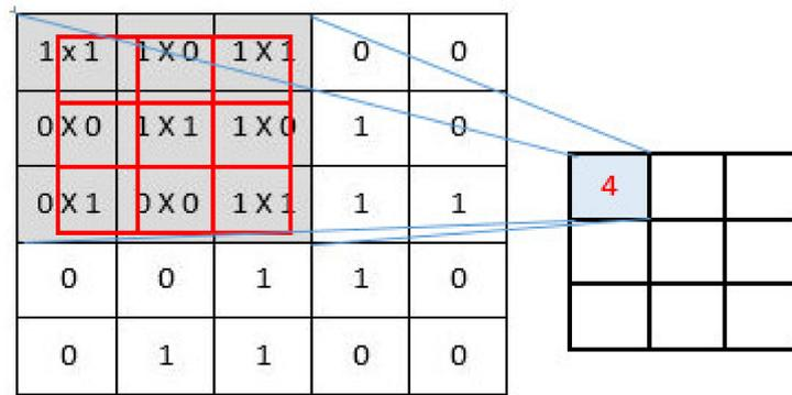
$$1 \times 1 + 1 \times 0 + 1 \times 1 + 0 \times 0 + 1 \times 1 + 1 \times 0 + 0 \times 1 + 0 \times 0 + 1 \times 1$$
