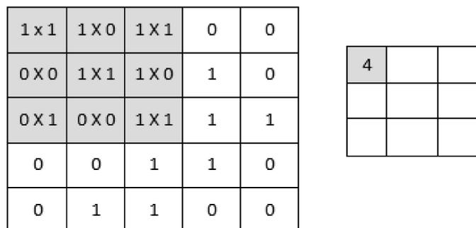
Figure 5. Calculation of filter slides over input image [8].
