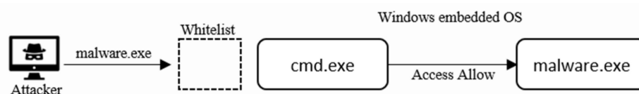
Figure 14. DAC-based whitelist security system.
