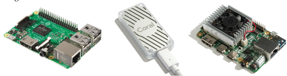
Figure 2. General-purpose embedded platforms and TPU-based platforms: RPi 4B (left), USB Coral TPU (center) and Coral Devboard (right).
