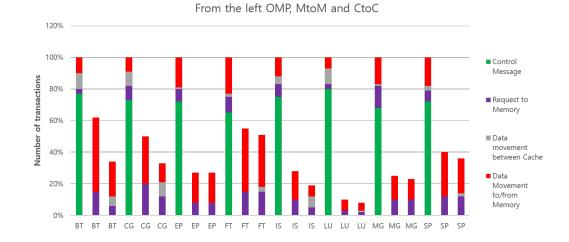
**Figure 15.** Total number of transactions on interconnection of all benchmarks for each architecture with different configurations.
