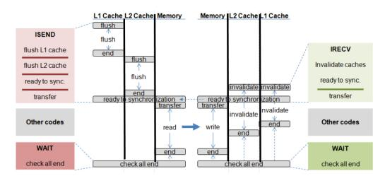
Figure 7. Non-blocking memory-to-memory transfer.
