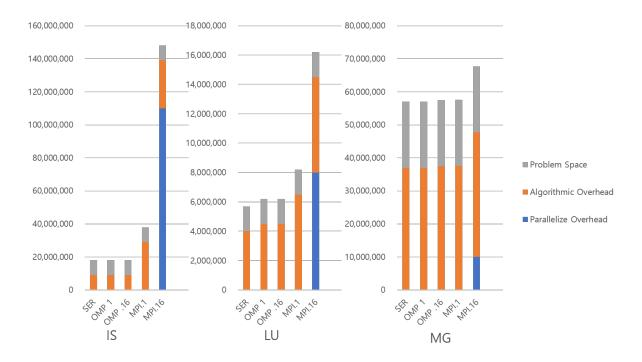
**Figure 2.** Categorization of parallel overheads in benchmarks (IS, LU and MG). Note that the SP benchmark is omitted because the characteristics of BT and SP benchmarks are very similar.
