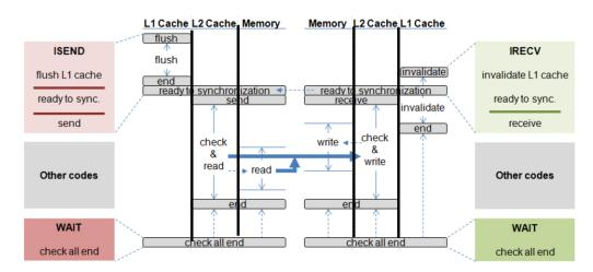
Figure 9. Non-blocking cache-to-cache transfer.
