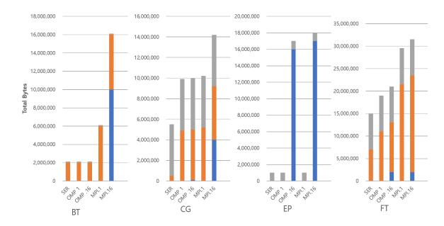
**Figure 1.** Categorizatio of parallel overheads in benchmarks (BT, CG, EP and FT). Note that the SP benchmark is omitted because the characteristics of BT and SP benchmarks are very similar.
