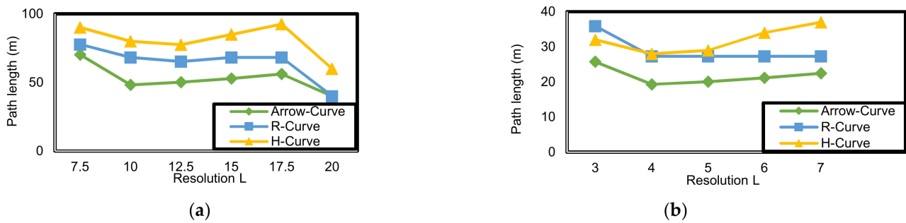
Figure 24. Path length (PL) corresponding to resolution (L) in Arrow-Curve model, R-Curve path model, and H-Curve (outdoor environment): (a) outdoor environment; (b) indoor environment.
