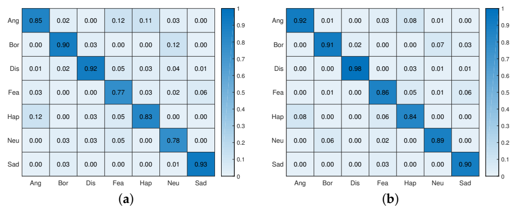
Figure 6. Confusion matrix with support vector machine (SVM) as classifier on EmoDB. (a) SVM [57], (b) multi-layer SVM.
