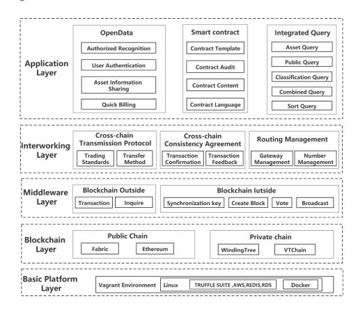
Figure 2. The layered architecture of the multi-chain.
