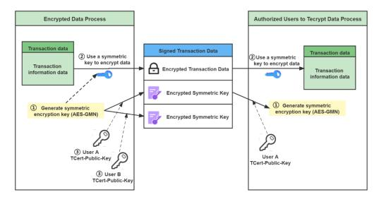
Figure 10. Data information encryption and decryption process.
