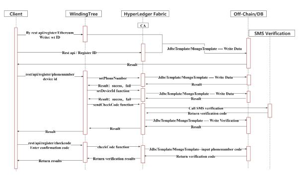
Figure 17. Execution process of user registration.
