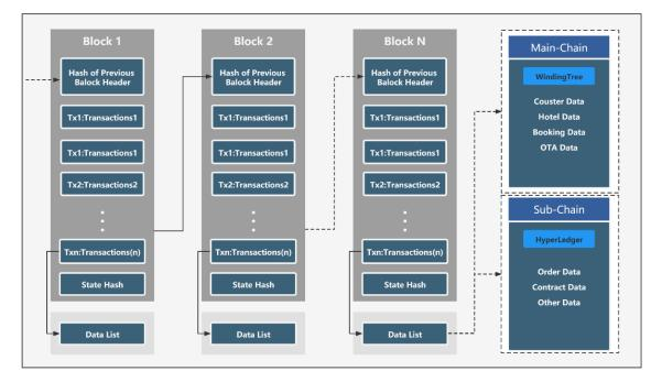
Figure 16. Block transaction information and structure.
