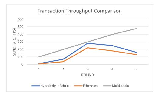
Figure 31. Comparison of three types of network transaction throughput performance.
