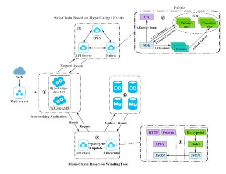
Figure 7. Overview of the multi-chain architecture.
