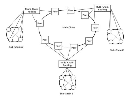
Figure 1. Overview of the multi-chain architecture.
