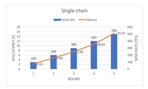
Figure 29. Network latency evaluation of single-chain architecture.
