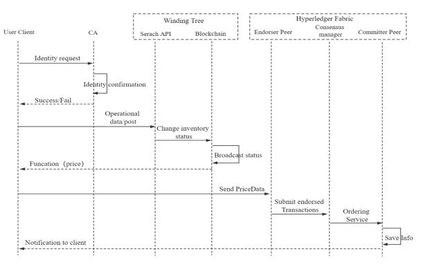
Figure 18. The transaction process of the proposed system.
