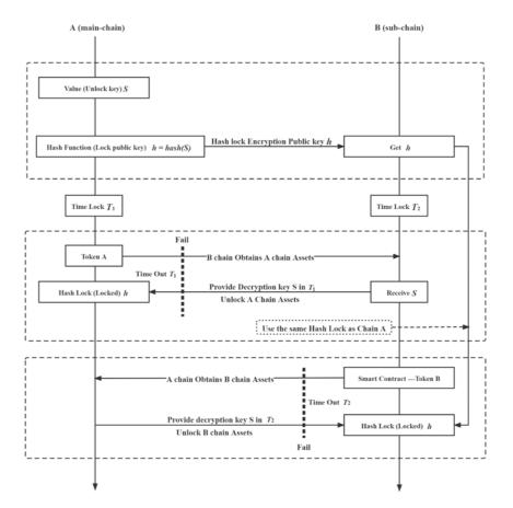
Figure 3. The principle of hash lock and hash time in cross-chain communication.
