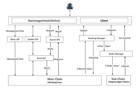
Figure 8. Interworking process based on multi-chain for secure tourism service.
