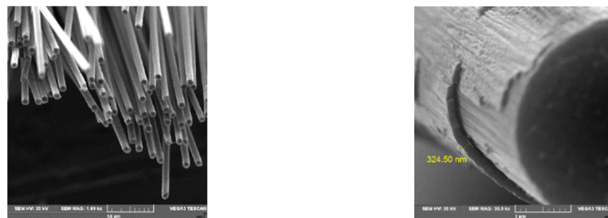
Figure 8. Metal-coated carbon fiber SEM measurement.
