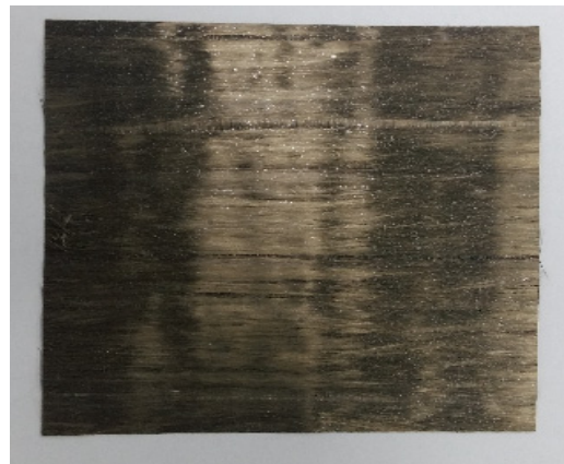
Figure 10. Metal-coated carbon fiber electromagnetic wave shielding film.
