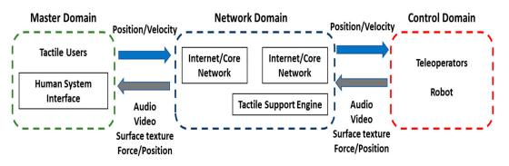
Figure 14. A generalized architecture of a wireless tactile internet system (adapted from [60]).
