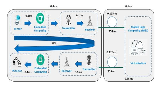
Figure 9. The various latency components of a typical TI system [41].
