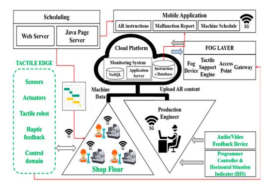
**Figure 16.** Integrating 5G and TI applications for integrated and adaptive AR maintenance and shop-floor rescheduling (adapted from [67]).
