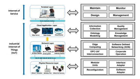
Figure 19. Hierarchical architecture of a smart factory (adapted from [71]).
