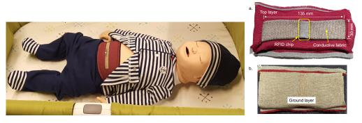
**Figure 1.** (**left**) A smart-fabric Bellyband and (**right**) Bellypatch can be integrated into wearable garments to enable wireless and passive biomedical monitoring in infants. (**a**) top and (**b**) bottom view of the Bellypatch.
