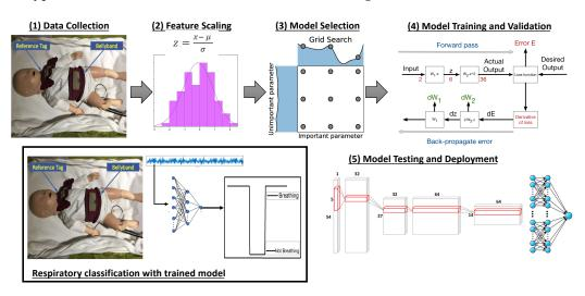
Figure 2. Design pipeline for respiratory classification using deep learning.
