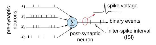
**Figure 7.** Integration of spike trains at the post-synaptic neuron from four pre-synaptic neurons in a spiking neural network (SNN). Each spike is a voltage waveform of ms time duration.
