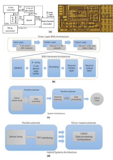
**Figure 18.** (a) Schematic diagram and optical image of RFID circuit [163] (Reprinted with permission from ref. [163]. Copyright 2022 INSTITUTION OF ENGINEERING AND TECHNOLOGY), (b) Diagram of BNN and hardware architectures, (c) Diagram of the system architecture of the natively flexible processing engine, and (d) Diagram of the system architecture and conceptual implementation of large-area sensor acquisition hybrid systems.
