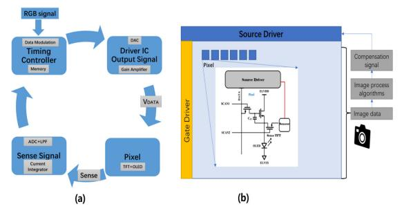
**Figure 7.** External compensation method: (**a**) Simplified block diagram. (**b**) External compensation approach.
