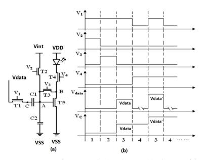
**Figure 4.** One-time detection method pixel circuit: (**a**) Schematic of the pixel circuit. (**b**) Timing diagram [112] (Reprinted with permission from ref. [112]. Copyright 2022 IEEE).
