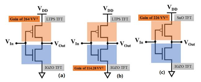
**Figure 12.** Inverter with LTPO: (a) Inverter of 264  $VV^{-1}$  gain, (b) Inverter of 114.28  $VV^{-1}$  gain, and (c) Inverter of 226  $VV^{-1}$  gain.
