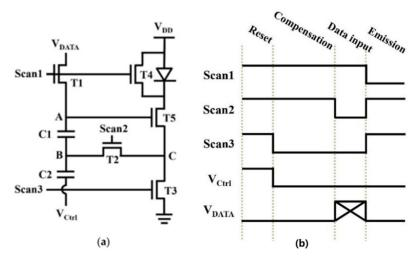
Figure 5. (a) Schematic of the pixel circuit. (b) Timing diagram [113].
