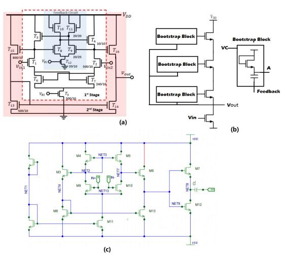
**Figure 14.** Amplifier of oxide-based TFT: (**a**) Transconductance-enhancement amplifier [157] (Reprinted with permission from ref. [157]. Copyright 2022 IEEE) and (**b**) Low noise amplifier. (**c**) LTPO amplifier.
