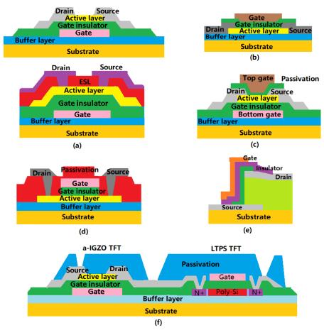
**Figure 1.** Typical device configurations of oxide semiconductors: (**a**) Back channel etch (BCE) and etch stop (ES) structure, (**b**) Top gate (TG) structure, (**c**) Dual gate (DG) structure, (**d**) Co-planar (CP) structure, (**e**) Vertical structure, and (**f**) Hybrid structure of LTPO.
