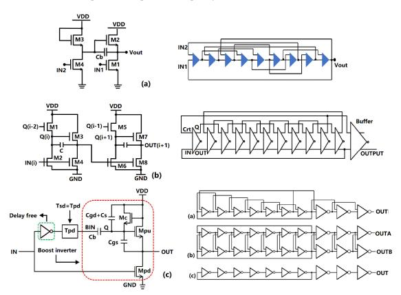
**Figure 13.** Oscillator with an optimized pseudo-CMOS inverter: (**a**) Diode-connected oscillator, (**b**) Pull-up control oscillator [79], and (**c**) Skewed delay oscillator [85].
