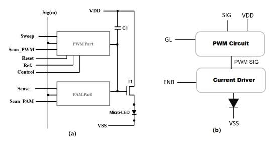
**Figure 10.** (a) PWM pixel circuit [52] (Reprinted with permission from ref. [52]. Copyright 2022 John Wiley and Sons). (b) Schematic diagram of current + PWM pixel circuit.
