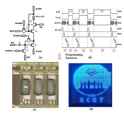
**Figure 9.** (a) Schematic of the proposed pixel circuit, (b) Timing diagram of the proposed pixel circuit, (c) Optical micrograph of the Micro-LED pixel circuit, and (d) Display of the Micro-LED [146] (Reprinted with permission from ref. [146]. Copyright 2022 IEEE).
