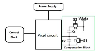
Figure 6. Schematic of the pixel circuit.
