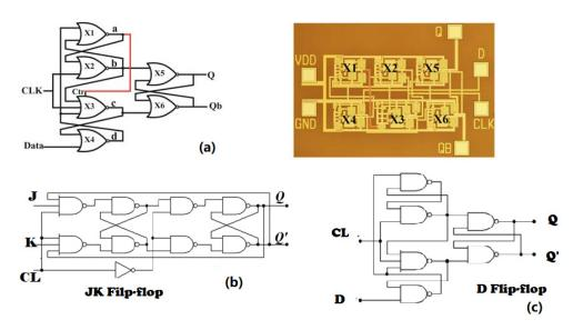
**Figure 17.** (a) Internal feedback control D flip-flop [164], (b) Complementary JK flip-flop, and (c) Complementary D flip-flop.
