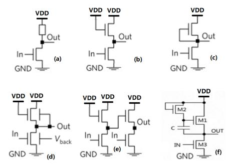
**Figure 11.** (**a**) Resistive-load logic inverter, (**b**) Diode-load logic inverter, (**c**) Zero-V<sub>gs</sub>-load logic inverter, (**d**) Dual-gate n-type diode-load logic inverter, (**e**) n-type diode-load pseudo-CMOS logic inverter, and (**f**) Bootstrapped NOT logic inverter.
