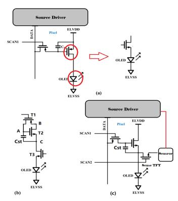
**Figure 3.** Degradation of TFTs and OLEDs and compensation technology: (**a**) Degradation in 2T1C circuit. (**b**) Internal compensation method. (**c**) External compensation method.
