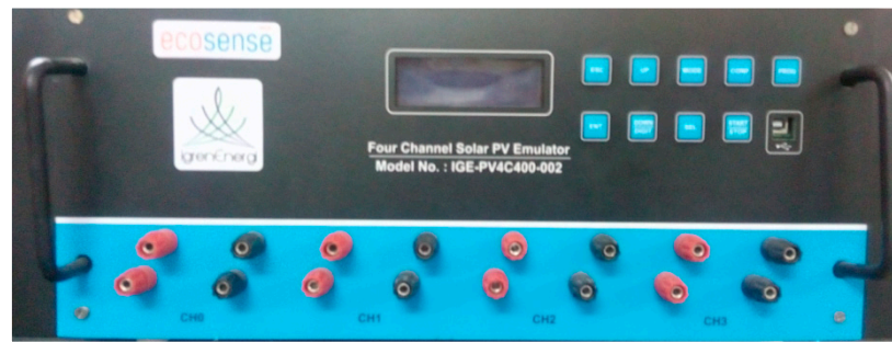
Figure 10. Solar PV emulator with four channels (CH1 to CH4).
