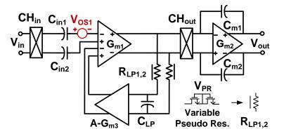
Figure 3. Schematic of the main path of CCIA with the block of proposed A-OCL.
