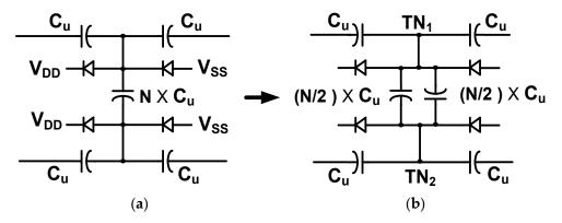
**Figure 5.** Schematic of the feedback T-network capacitor. (**a**) Conventional configuration; (**b**) modified configuration for symmetrical parasitic behavior.
