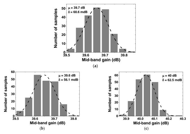
**Figure 11.** Monte Carlo simulation results of the mid-band gain of the proposed CCIA for different values of  $V_{DD}$ : (a)  $V_{DD} = 1 \text{ V}$ , (b)  $V_{DD} = 0.9 \text{ V}$ , and (c)  $V_{DD} = 1.1 \text{ V}$ .
