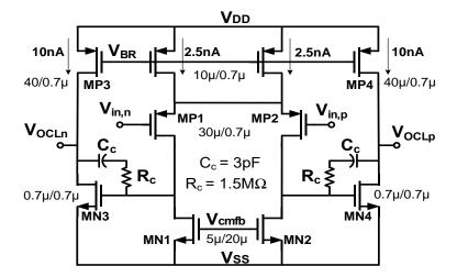
Figure 7. Schematic of the two-stage OTA G<sub>m3</sub> in A-OCL.
