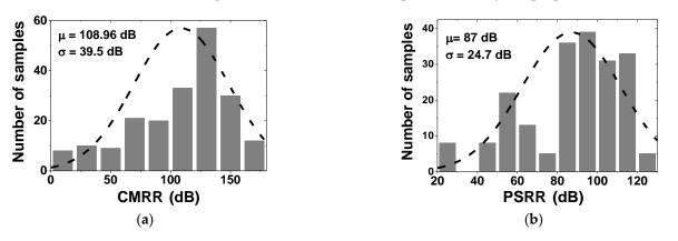
**Figure 13.** Monte Carlo simulation results of the proposed CCIA: (**a**) Common mode rejection ratio CMRR; (**b**) power supply rejection ratio PSRR.
