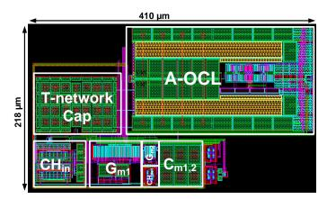
Figure 8. Chip layout of the proposed CCIA.
