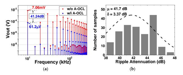
**Figure 14.** Simulation results of the proposed CCIA: (**a**) Spectrum output voltage with and without A-OCL; (**b**) Monte Carlo simulation of the attenuation ripple.
