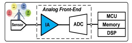
Figure 1. Block diagram of a biopotential acquisition system.
