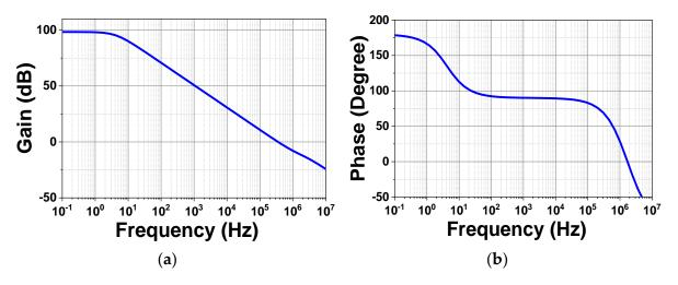
**Figure 9.** Open-loop simulation results for gain (**a**) and phase (**b**) versus frequency of main path amplifier with active A-OCL.
