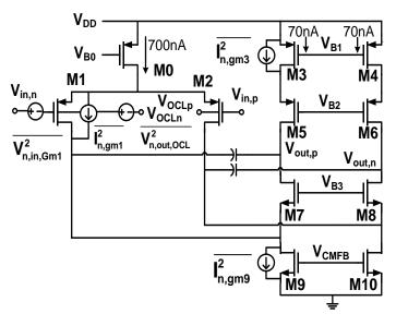
Figure 6. Schematic of the folded cascode op amp using buck control with its noise sources.
