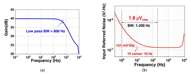
**Figure 10.** The simulation results of the proposed CCIA: (**a**) the frequency response; (**b**) the input referred noise.
