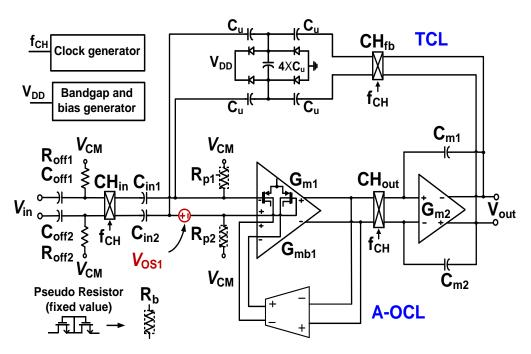
Figure 2. Schematic of the proposed CCIA using A-OCL.  $C_{in1,2} = 2 \text{ pF}$ ,  $C_{fbeq1,2} = 20 \text{ fF}$ ,  $C_{m1,2} = 1.5 \text{ pF}$ .
