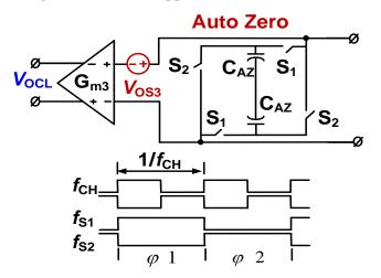
Figure 4. Schematic of the auto-zero offset A-Gm3 and timing diagram.
