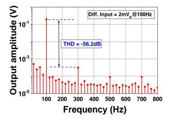
Figure 15. Linearity verification by applying FFT analysis of output voltage with 100 Hz input frequency.
