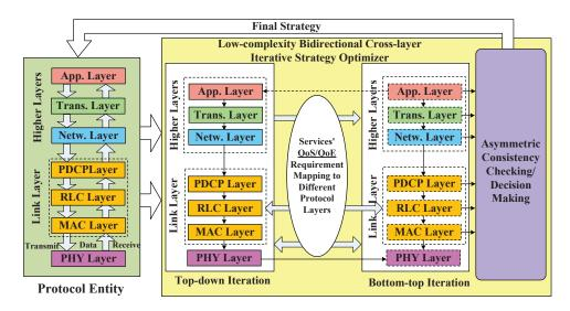
**Figure 6.** Tightly coupled cross-layer framework with service-awareness achieved via bidirectional iterative strategy optimization (using the typical architecture of a protocol stack in 3GPP as an example).
