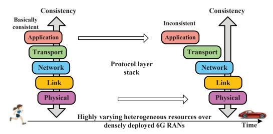
**Figure 5.** Inconsistent responses to the highly varying heterogeneous network status caused by the loosely coupled protocol stack.
