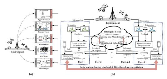
Figure 4. The model of the distributed AI: (a) the vertical dimension; (b) the horizontal dimension.
