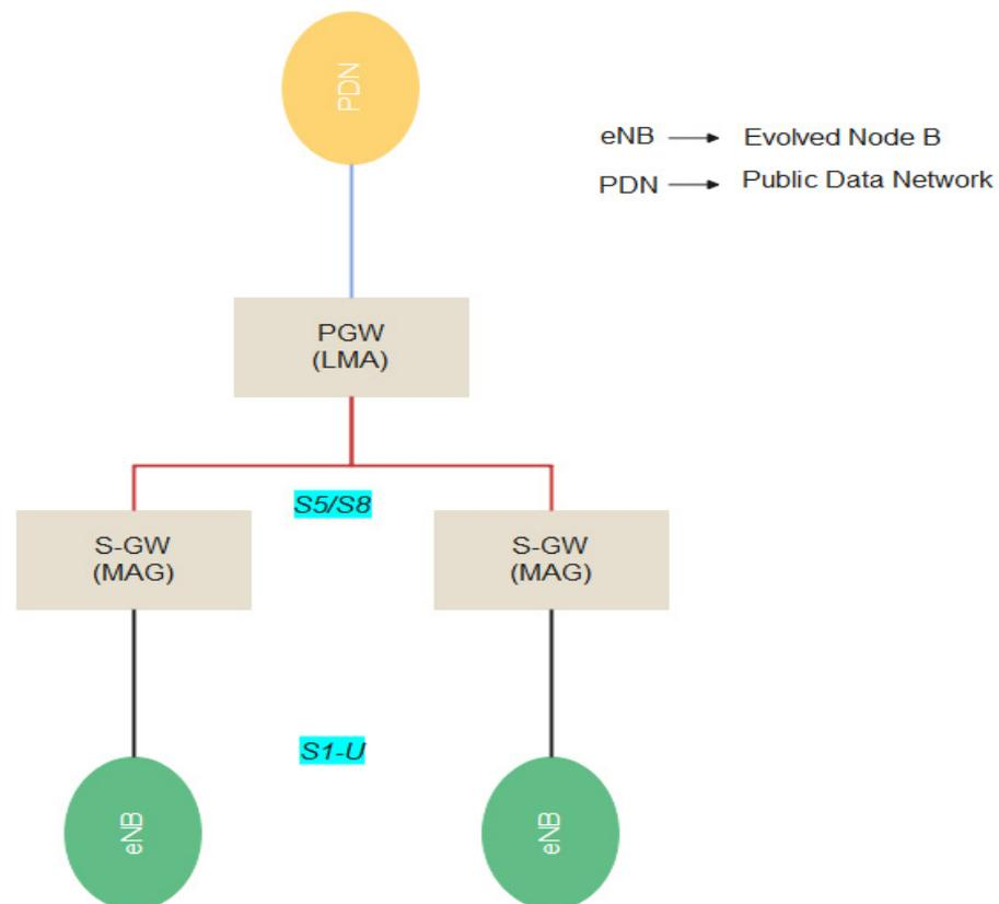
**Figure 5.** PMIPv6 in the 3GPP EPC system.
