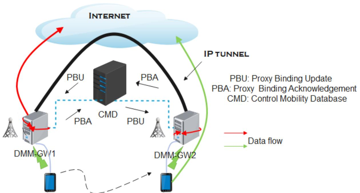
Figure 7. PMIPv6-based DMM.
