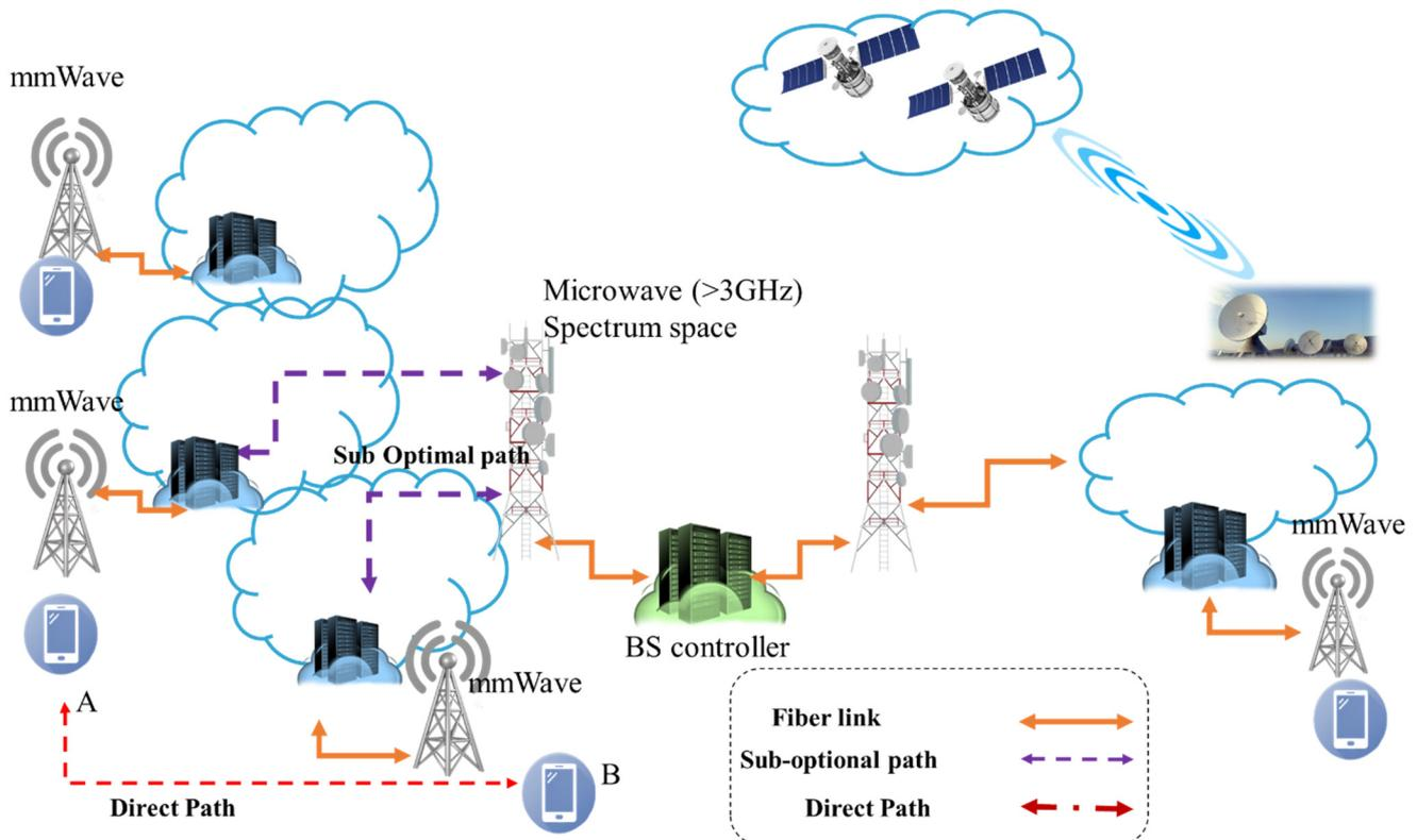
**Figure 6.** A distributed network that places content servers in the access network.
