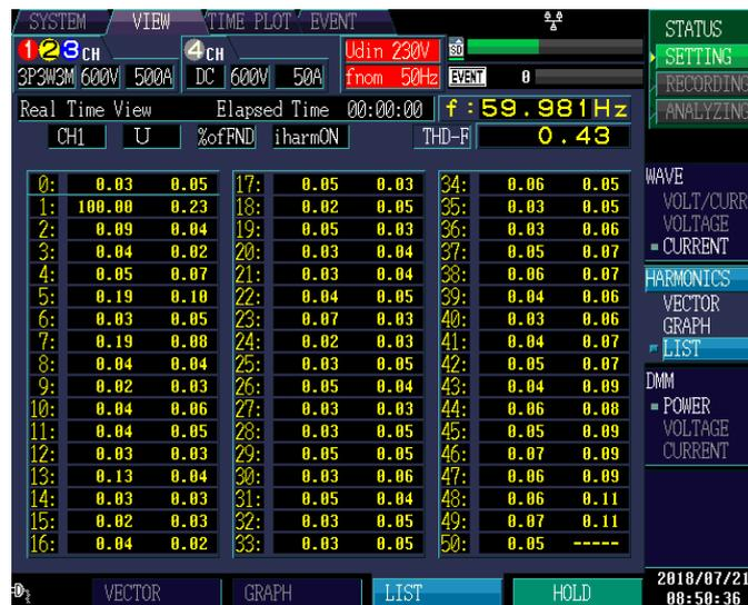
Figure 15. Harmonic components of the line currents up to the 50th were obtained by three-phase, three-wire connection for the operating conditions in Figure 14a.
