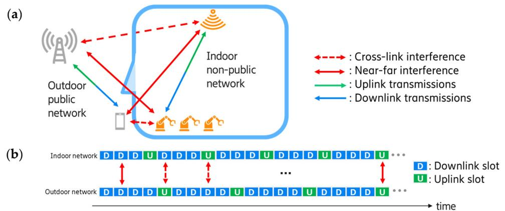
**Figure 1.** Illustration of interference situation caused by coexisting indoor and outdoor networks. (a) Interference links between base stations and UEs of indoor and outdoor networks when different TDD patterns are selected. (b) Different TDD patterns used in the indoor network compared to the outdoor network result in both near-far interference and cross-link interference.
