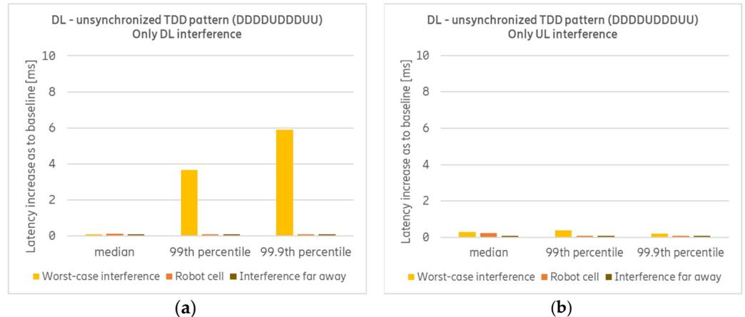
**Figure 8.** Increase in DL latency compared to the respective baseline for unsynchronized TDD pattern (indoors: DDDDUDDDUU, outdoors: DDDDU) and different indoor/outdoor UE deployment locations. (a) Result for only DL interference (near–far interference). (b) Result for only UL interference (cross-link interference).
