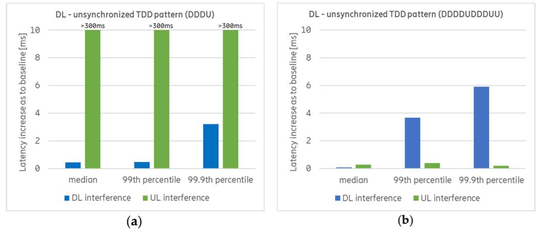
**Figure 5.** Increase in DL latency compared to its baseline for unsynchronized TDD pattern. (a) Indoor TDD pattern DDDU and outdoors DDDDU are configured. (b) Indoor TDD pattern DDDDUDDDUU and outdoors DDDDU are configured.
