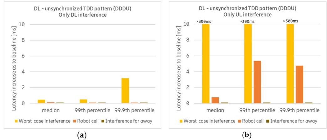
**Figure 7.** Increase in DL latency compared to baseline for unsynchronized TDD pattern (indoors: DDDU, outdoors: DDDDU) and different indoor/outdoor UE deployment locations. (a) Result for only DL interference (near–far interference). (b) Result for only UL interference (cross-link interference).
