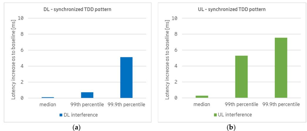
**Figure 3.** Increase in DL (a) and UL (b) latency compared to their respective baselines for synchronized TDD pattern (DDDDU) used by the indoor and outdoor networks.
