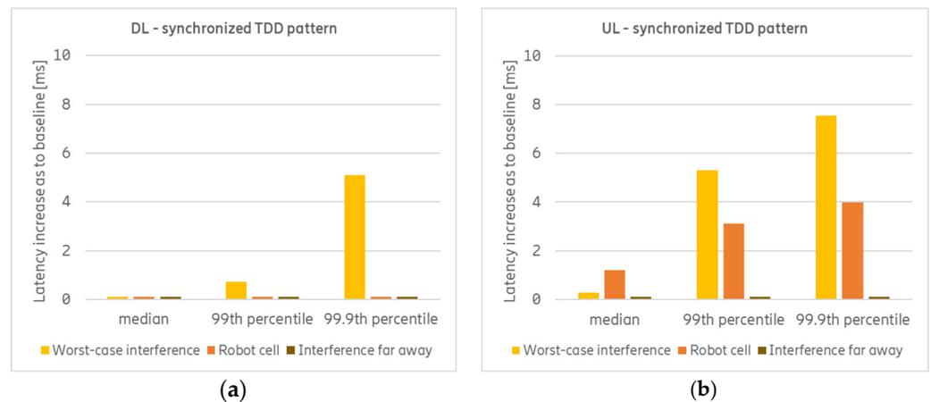
**Figure 4.** Increase in DL (a) and UL (b) latency compared to their baselines for synchronized TDD pattern of DDDDU with different indoor/outdoor UE deployment locations.
