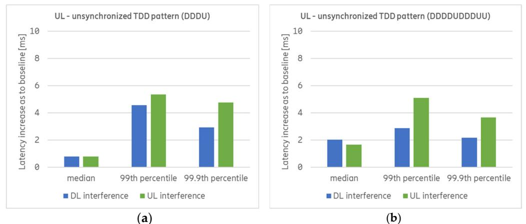
**Figure 6.** Increase in UL latency compared to its baseline for unsynchronized TDD pattern. (a) Indoor TDD pattern DDDU while outdoors DDDDU are configured. (b) Indoor TDD pattern DDDDUDDDUU and outdoor DDDDU are configured.
