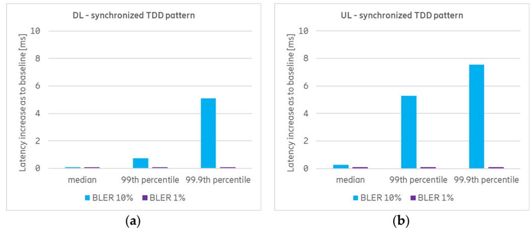
**Figure 9.** DL (a) and UL (b) latency increase compared to their baseline for synchronized TDD pattern when using different BLER targets in the worst-case deployment setup.
