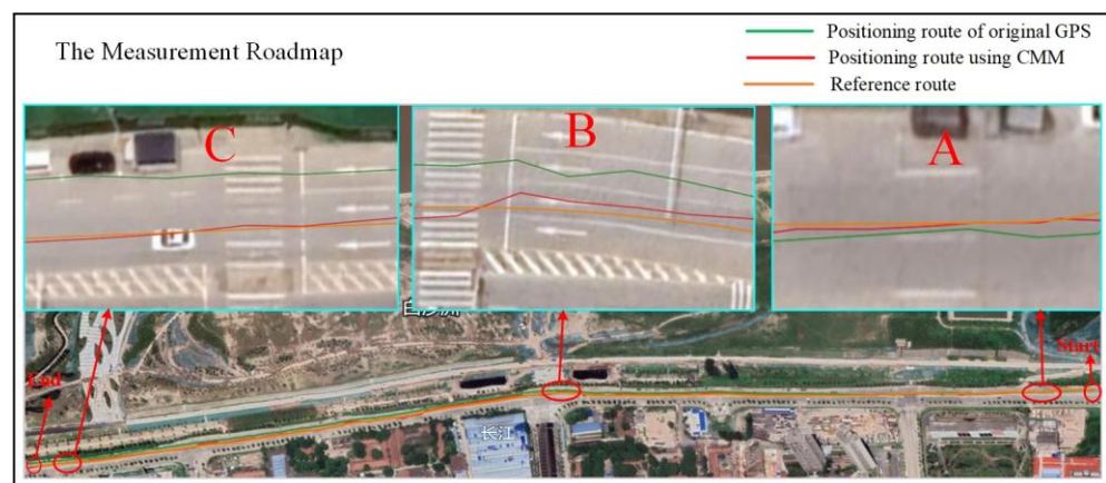
Figure 13. Dynamic positioning result reproduced on Google Earth.
