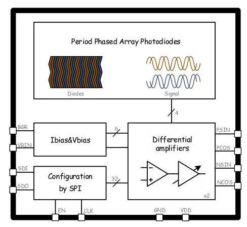
Figure 2. Framework of the phased array detector chip.
