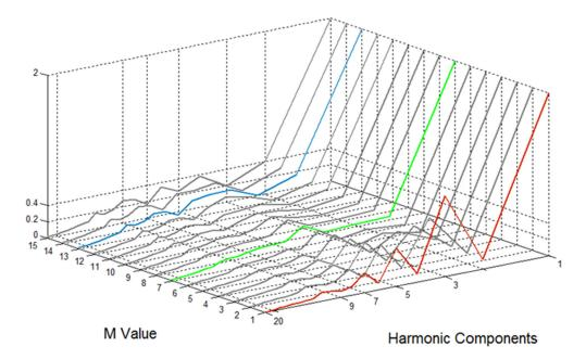
Figure 4. The effect of the number of detectors on harmonic components.
