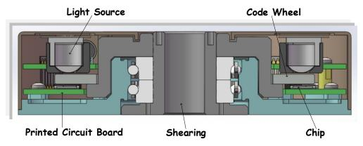
Figure 1. Phased array optoelectronic encoder structures.
