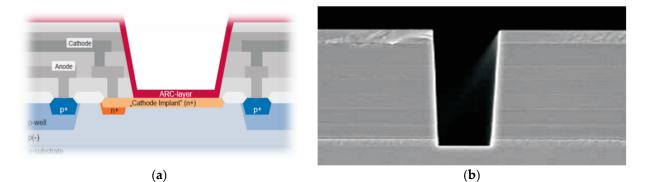
**Figure 11.** High-speed p-i-n photodiode structure in X-FAB process library: (**a**) section of the structure; (**b**) optical window etching.
