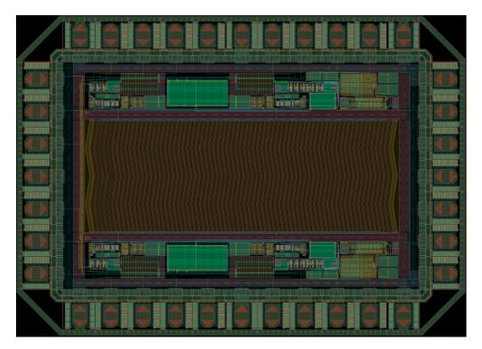
Figure 6. Layout of the phased array detector chip.
