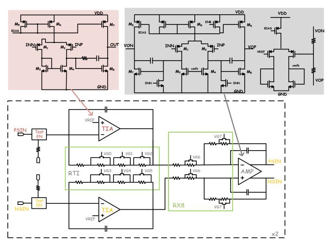
adjustment is reserved. By adjusting the resistance value, the gain of the amplifier can be adjusted to a certain extent.
