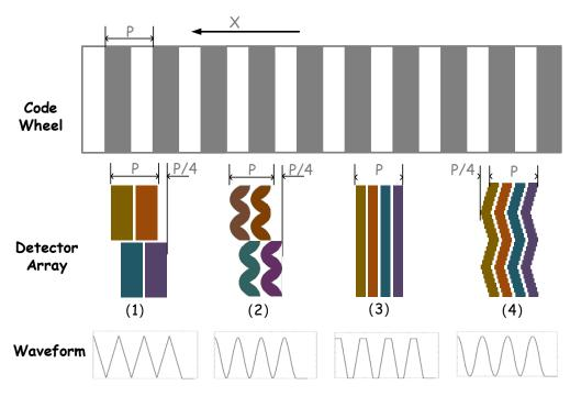
Figure 3. Arrangements of different phased arrays.
