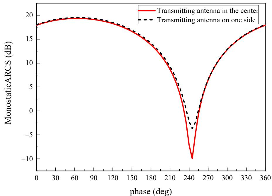
**Figure 7.** The Minimum ARCS of the target on the direction the aircraft is facing when the echo cancellation antenna is placed on one side or in the center.
