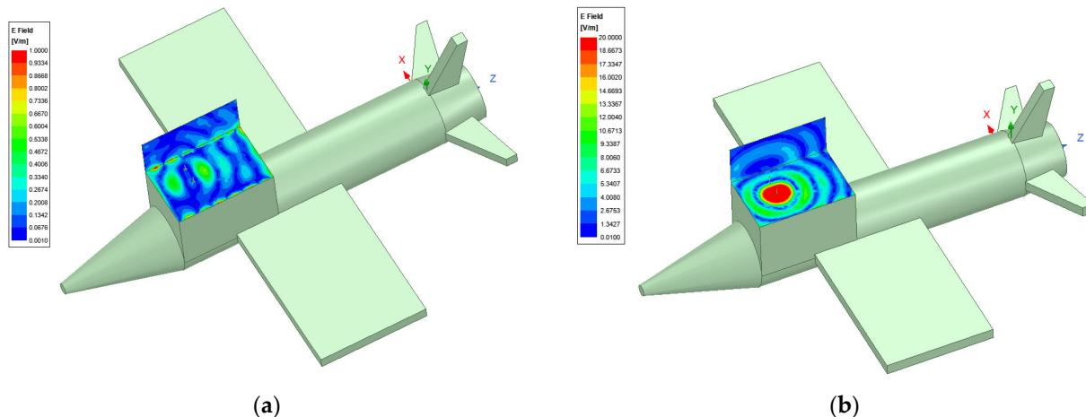
**Figure 4.** (a) Electromagnetic field around the antenna system before the echo cancellation; (b) Electromagnetic field around the antenna system after the echo cancellation.
