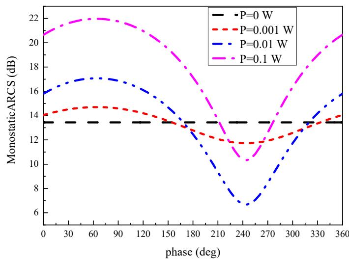
**Figure 5.** ARCS of the target at antenna transmit power of 0.001 W, 0.01 W, 0.1 W and 0 W.
