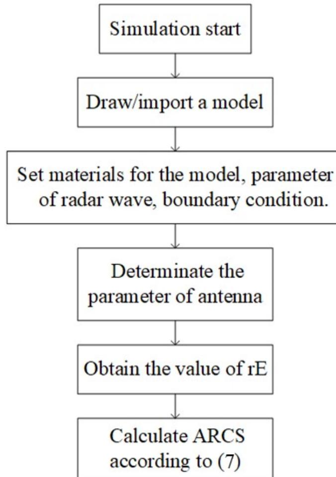
**Figure 2.** The entire flow diagram of ARCS simulation procedures.
