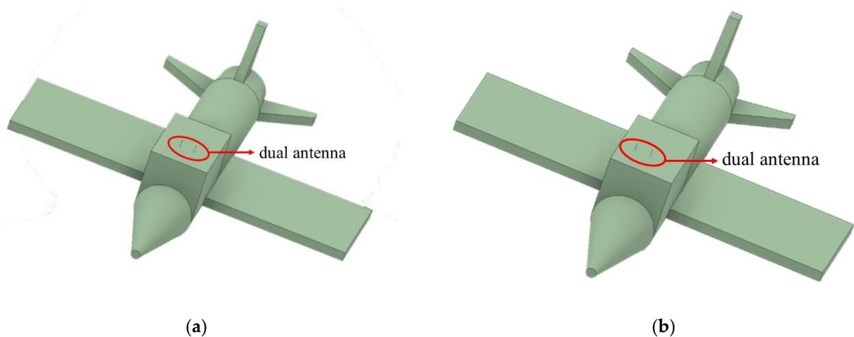
**Figure 6.** (a) 3D-model of the antenna placed on both sides of the target; (b) 3D-model of the echo cancellation antenna placed in the center of the target.
