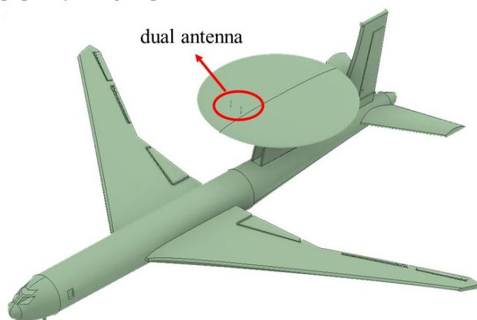
**Figure 9.** 3D-model of the aircraft with the dual antenna structure.
