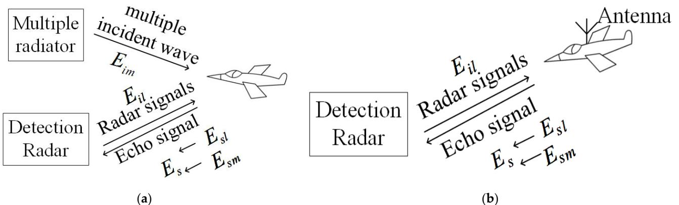
**Figure 1.** Two different ARCS cases (a) target illuminated by radar and multiple radiators (b) target illuminated by radar and antenna.
