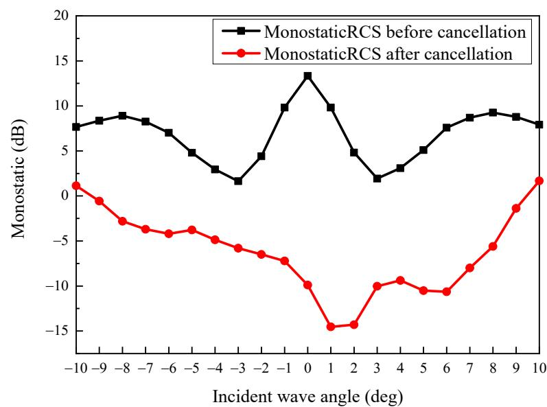
**Figure 8.** Minimum ARCS for targets with azimuths in the range of  $-10$  degrees to  $10$  degrees.
