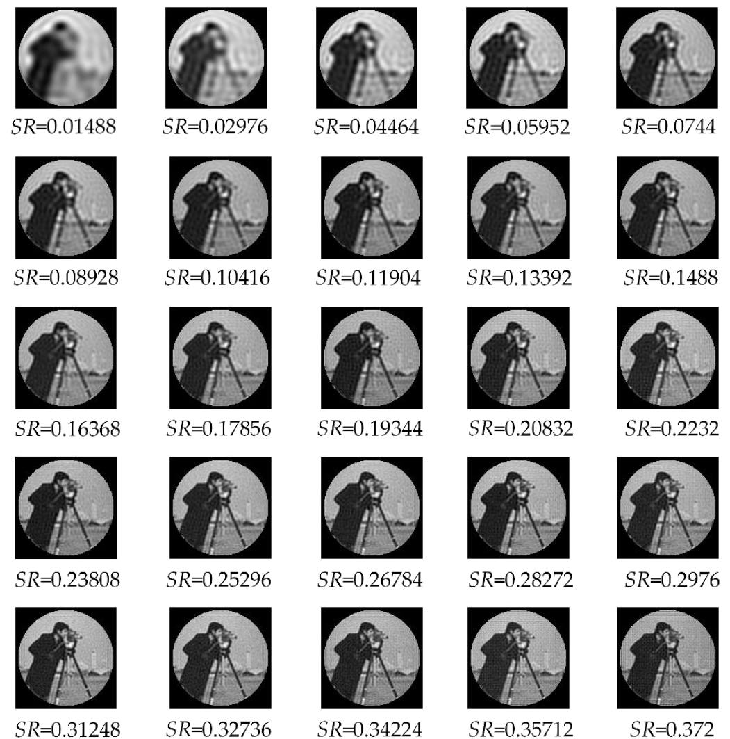
Figure 2. Reconstructions of different sampling ratios by Zernike single-pixel imaging.
