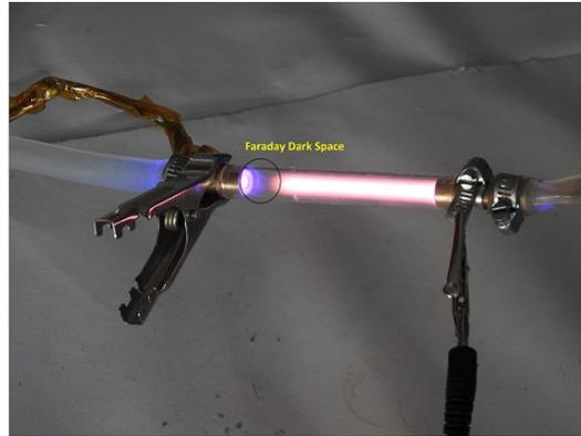
**Figure 9.** Experimental demonstration of DC glow discharge.
