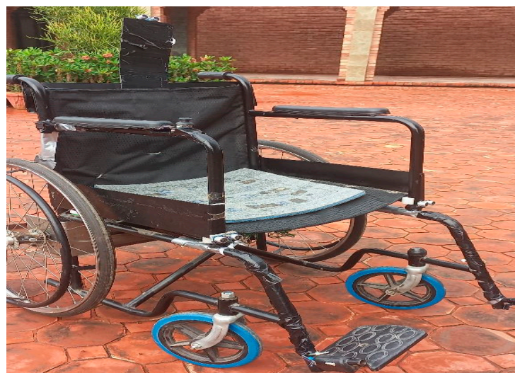
Figure 9. Manual Wheelchair is converted to multi-mode electric wheelchair by installing designed conversion kit.
