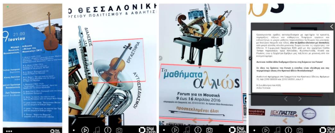
Figure 7. Access to the camera of the handheld device and the AR functions. In the left image, the recognition of a marker (text) and the display in 3-D of a cello. In the next image, the marker (image) recognized in an analogue poster, and in the last two images, the marker (text) recognized and display of additional informative text.
