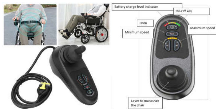
Figure 12. Manual control of motorized wheelchair.
