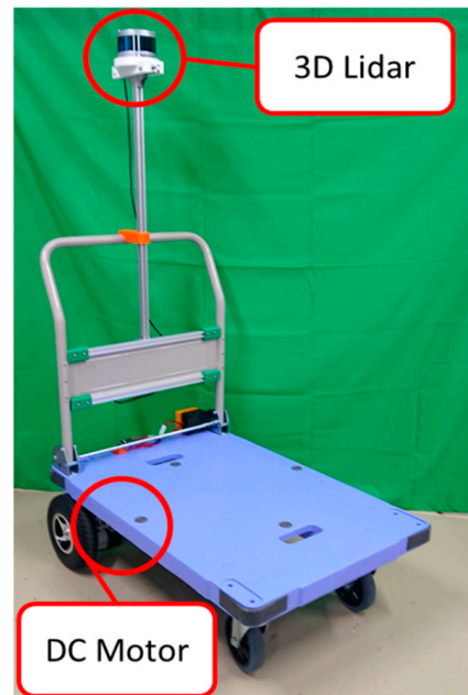
Figure 2. Modified trolley cart that served as the automated vehicle in this study.
