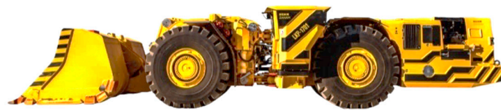
Figure 2. Load-haul-dumping (LHD) vehicle for underground operations [38].
