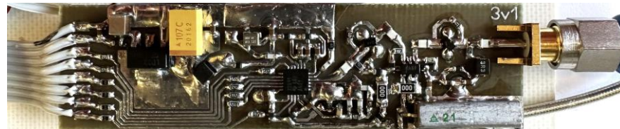
Figure 7. Photograph of the PLL 1 prototype. The coaxial resonator is clearly visible in the lower right corner. This image demonstrates the simplicity of the proposed frequency sweep topology. Implemented on a single-layer PCB without vias, this design is well-suited for rapid prototyping. Notably, this approach translates to a cost-effective solution for industrial applications.
