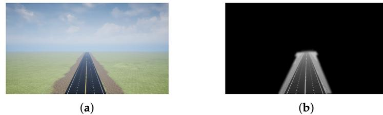
**Figure 19.** The processed image that is fed into ORB-SLAM2: (a) original image (b) processed image.
