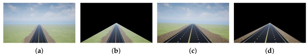
**Figure 6.** Examples of cropped images: (a) zero  $\phi$ , original image (b) zero  $\phi$ , cropped image (c) slight  $\phi$ , original image (d) slight  $\phi$ , cropped image.
