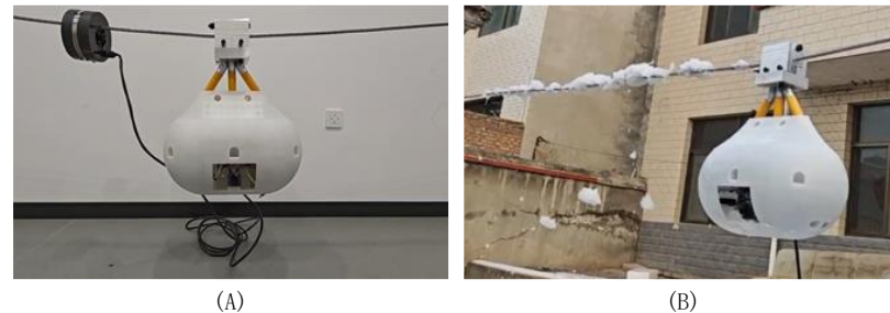
Figure 1. Suspended intelligent vibration de-icing robot: (A) static display, (B) deicing process.
