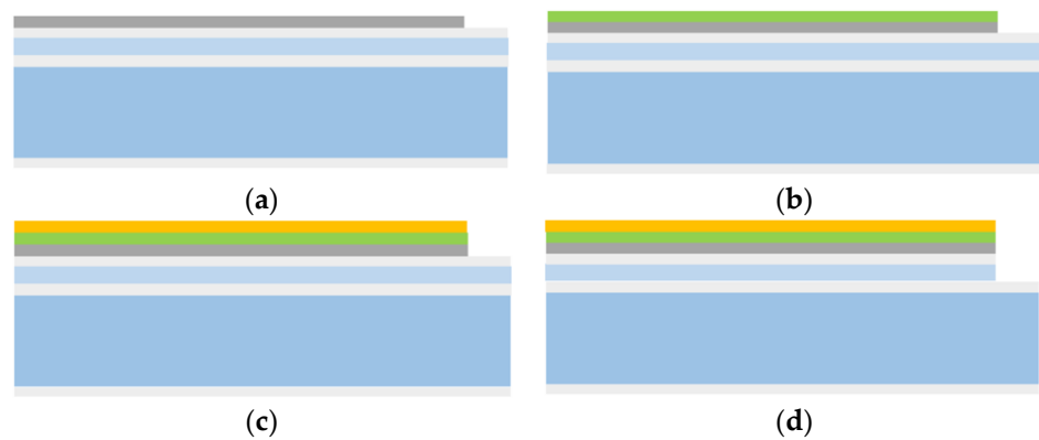
Figure 3. The process masks for one MEMS device: (a) Mask 1—bottom electrode patterning; (b) Mask 2—piezoelectric configuration; (c) Mask 3—top electrode patterning; (d) Mask 4—cantilevers configuration; (e) Mask 5—cantilevers release; (f) overlaying of the five masks.
