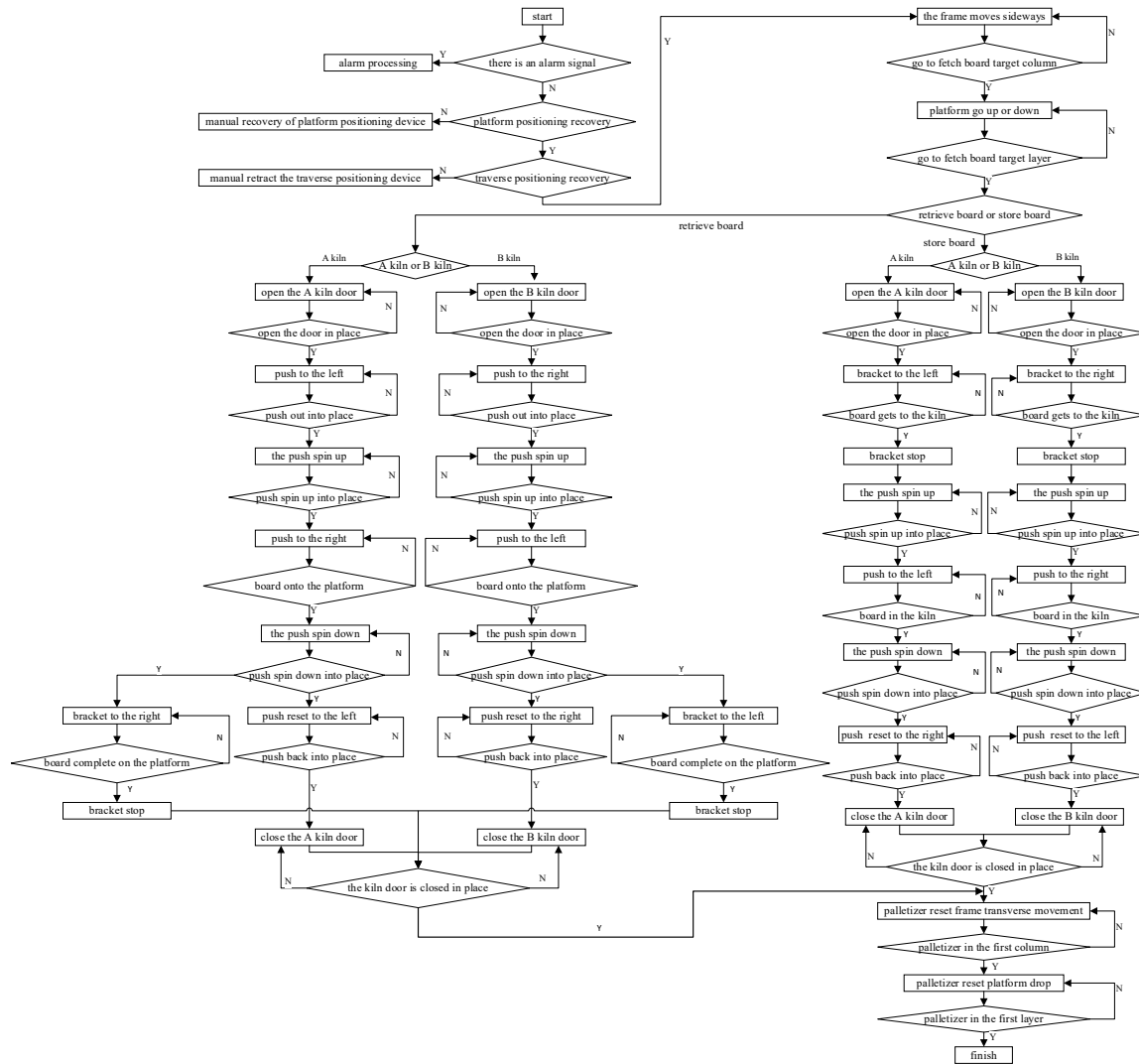
Figure 7. Board retrieval and storage control program flowchart.
