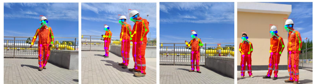
Figure 9. Application result of HR-YOLO for outdoor scene detection. The colored line segments in the figure are the human pose estimation lines corresponding to the 18 key points.
