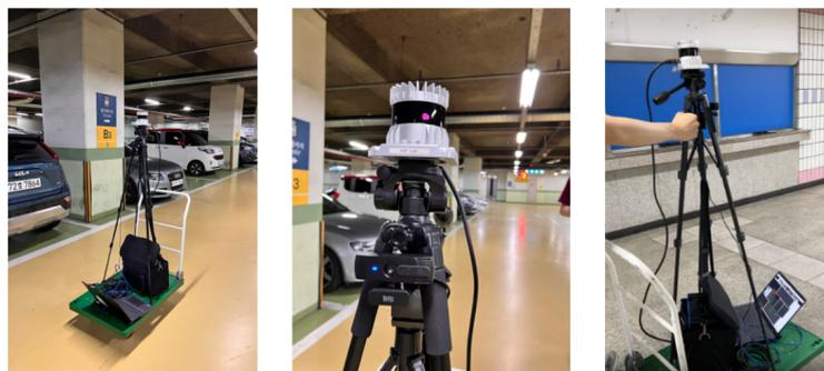
**Figure 3.** Experimental platform with a 64-channel 3D laser scanner.
