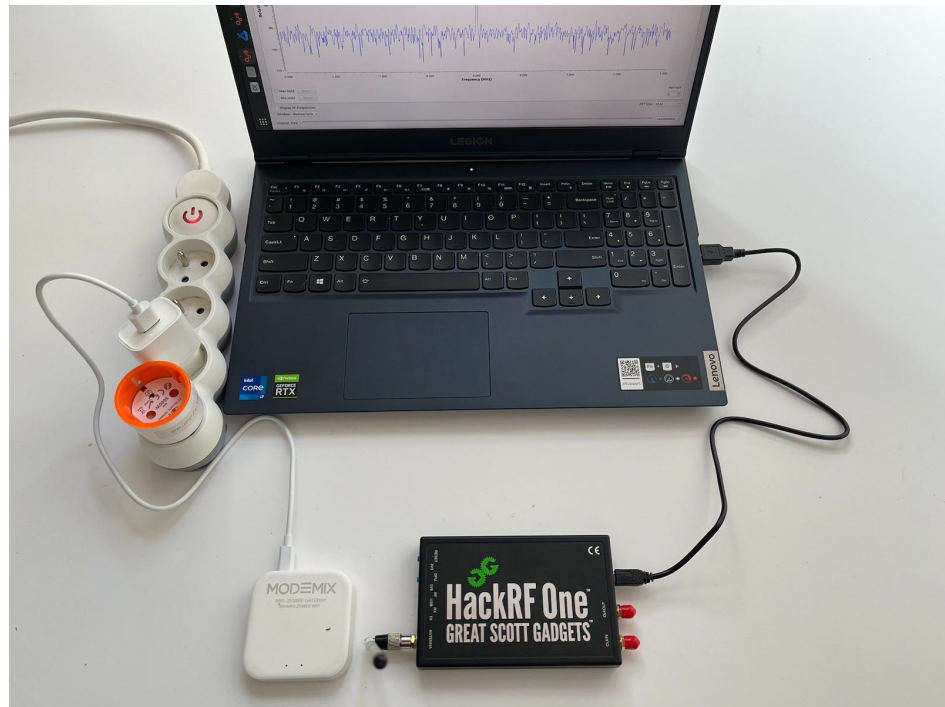
Figure 17. Lab realization of the setup from Figure 16.
