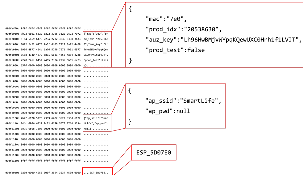
Figure 11. Analysis of memory area from 000fb000 to 000fb17f in Gosund SP111 firmware.
