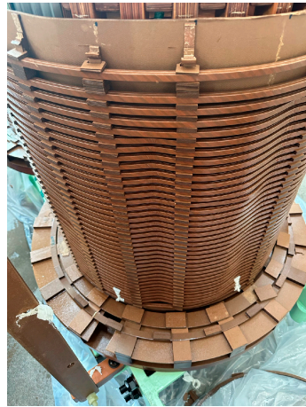
Figure 13. The deformed winding.
