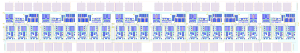
Figure 8. Layout of the designed fourth-order reconfigurable Gm-C filter, with a occupied silicon area of 1137 \mu\text{m} \times 199 \mu\text{m} ( 0.23 \text{ mm}^2 ).
