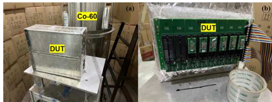
Figure 3. The irradiation platform (a) and the 7T SOI SRAMs under test (b) of the TID experiment.
