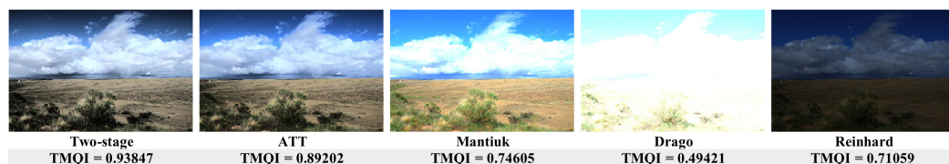
Figure 2. TMQI-based comparison on the Funt dataset across five tone mapping methods.
