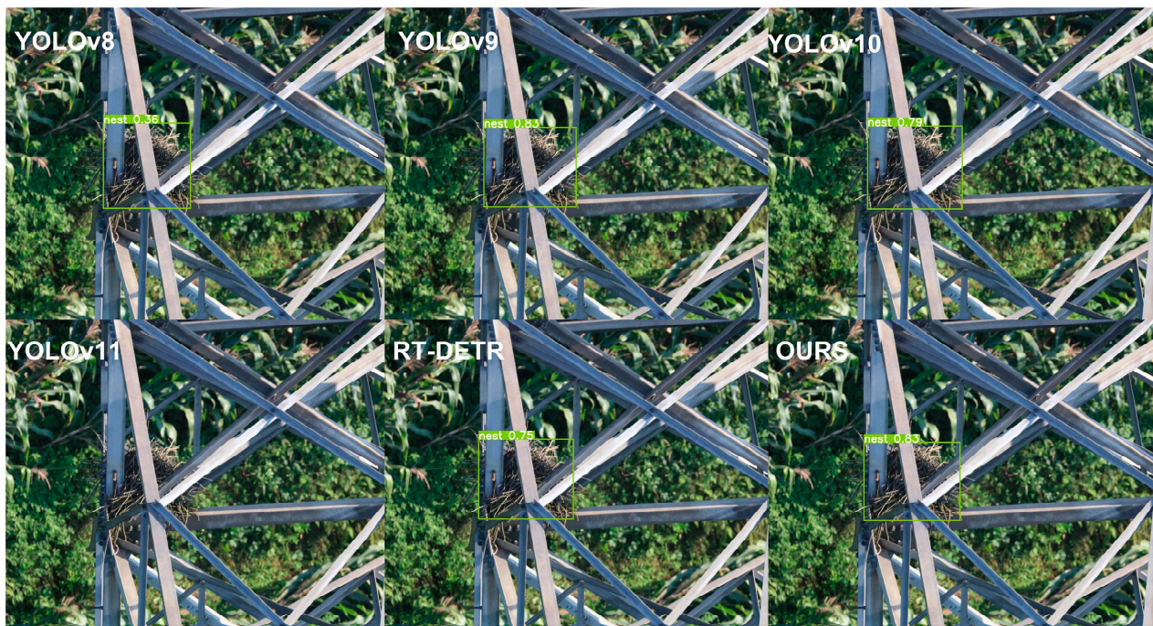
Figure 11. Bird nest inspection visualization results (YOLOv8, YOLOv9, YOLOv10, YOLOv11, RT-DETR, PLD-DETR).
