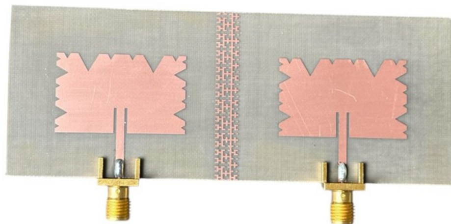
Figure 36. Fabricated antenna with fractal geometries.
